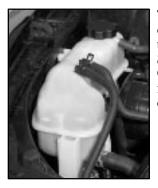
The surge tank is located on the passenger's side of the engine compartment. See "Engine Compartment Overview" in the Index for more information on location. The vehicle must be on a level surface. When your engine is cold, the coolant level should be at the FULL COLD mark.
